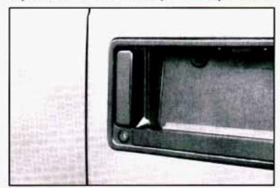
To open the rear doors from the outside, open the right rear door first. Grasp the handle and pull the door open.
